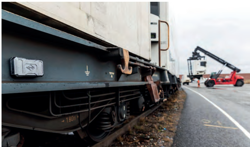
The RMD Performance Monitoring Unit mounted on an intermodal wagon.
